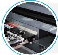
High-Speed Carriage on Dual Guide Rails with Brake Motor Positioning — Guarantees Precise and Reliable Stopping Accuracy.
